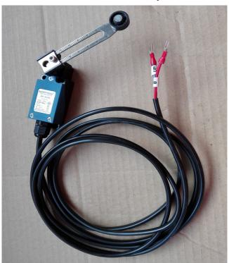
The limit switch is installed on the post anti-hoist cylinder limit, The wiring diagram in the electrical box inside is the number 8 and the other one of the terminals which showing "up".
