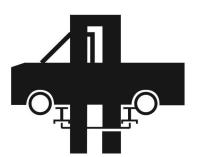
Ensure the position of the vehicle is safe and correct, when the vehicle left the ground.
